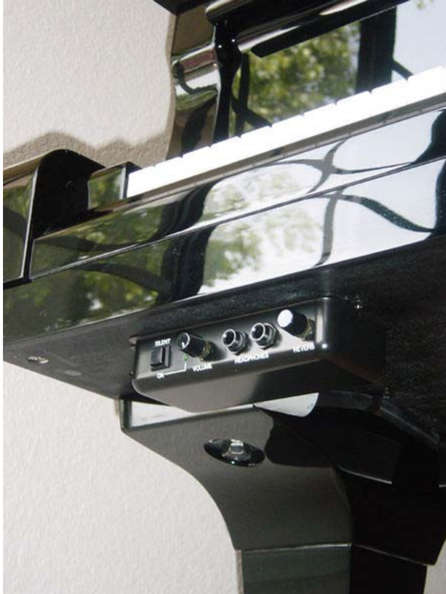
Sequencer control unit of Yamaha Disklavier Mark III
