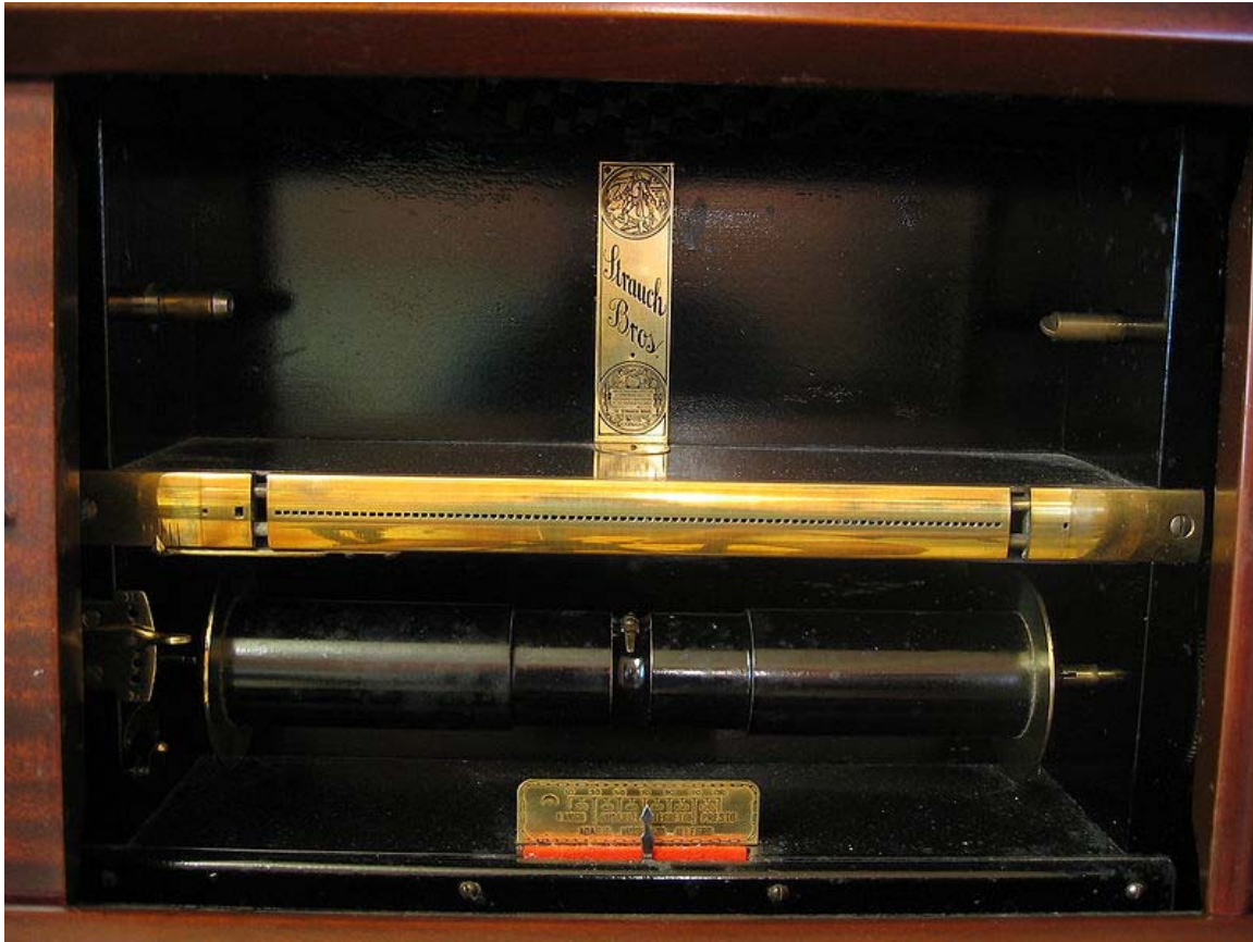
Horizontal row of tracker tubes detects music roll holes
