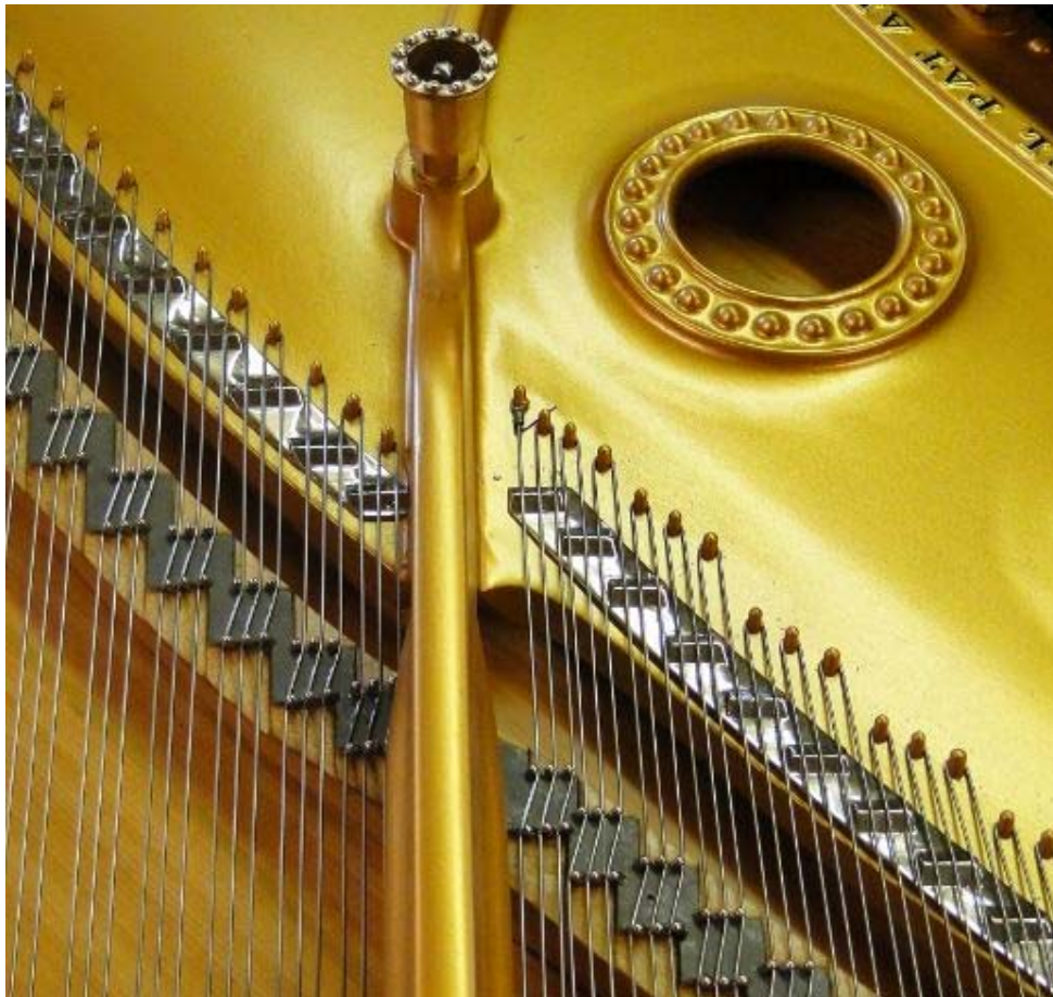
Duplex scaling of an 1883 Steinway Model 'A'. From lower left to upper right: main sounding length of strings, treble bridge, duplex string length, duplex bar (nickel-plated bar parallel to bridge), hitchpins, plate strut with bearing bolt, plate hole.
